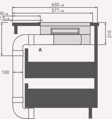
**A** - POSITIE AANSLUITING SNOER AFZUIGING EN KOKPLAAT
